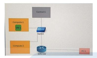
Virtual machine VM-1 is spawned on compute node Compute-1. VM-1 is not able to ping PC-1, which is located outside of the SDN cloud. You want to run packet captures to trace the packet initiated by VM-1 towards PC-1. Which three interfaces would you use to accomplish this task? (Choose Three)
